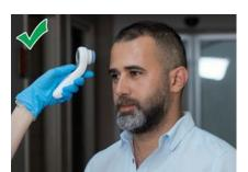
Figure 1: Correct Use – Forehead unobstructed, and NCIT held perpendicular to front of forehead; and used at distance identified in manufacturer's instructions.
